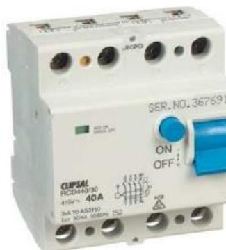
2) **RCD (Residual Current Device)** - This is the device that detects earth leakage. THIS IS THE DEVICE THAT TRIPS IF YOU ARE GETTING ELECTROCUTED. It shows that there is faulty wiring onboard and can be potentially life threatening - Must be investigated by a marine 240v electrician.
